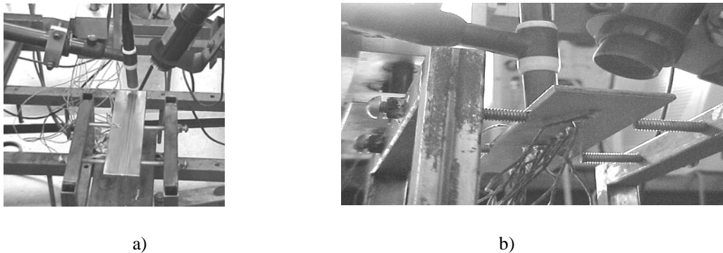
Figure 2. Experimental apparatus: a) view of welding torch; b) view of thermocouple attaching.
